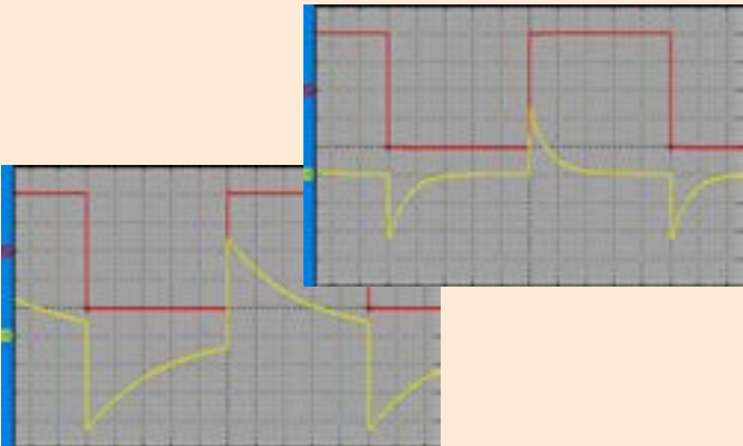
Changing the cut-off frequency also changes the step response.
